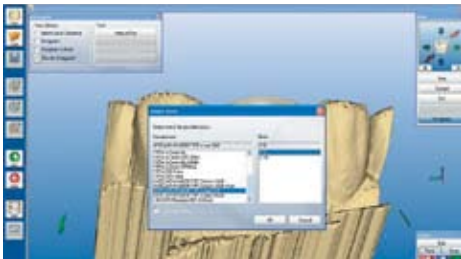
Fig. G The material block is selected from among a list of available materials
