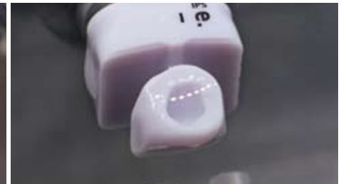
Fig. I After milling, the crown coping is attached to the remaining block by a sprue.
