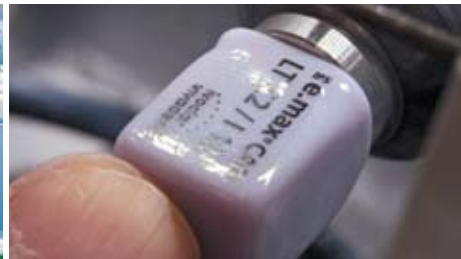
Fig. H The material block is secured into the milling chamber, and milling is commenced.
